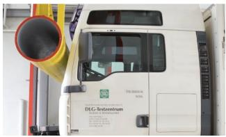
**ROPS tests on machines of up to 100 tonnes:** The DLG Test Center has two ROPS testing rigs that offer facilities for testing cabs on heavy-duty machinery with a max. weight up to 100 tonnes by applying forces of approx. 1,500kN horizontally and 2,000kN vertically.
